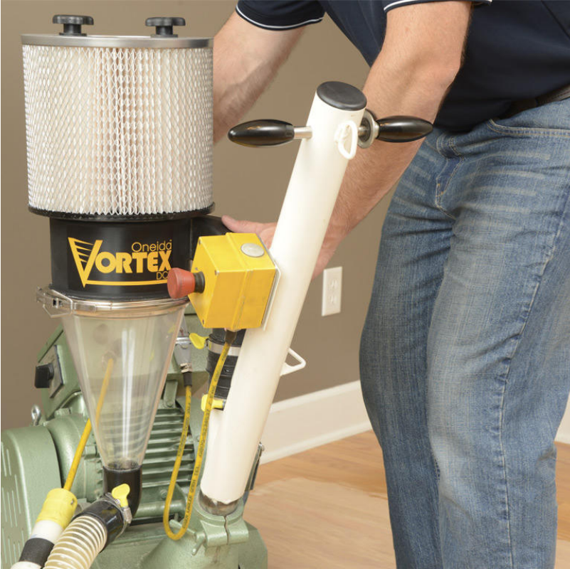
Sealed collector on the machine · HEPA at the shoe
